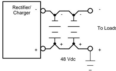
Figure 1: The traditional connection of one rectifier (battery charger) with a group of batteries. The rectifier provides current to supply the load plus charge the batteries.
