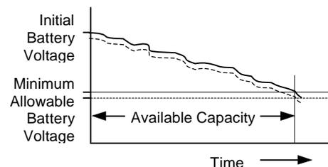
Figure 5: Same diagram as Figure 1, except 0.7 Vdc drop from series connected blocking diode on each battery string. The underlying battery capacity remains unchanged as long as the logic is programmed to consume power to 0.7 Vdc below the previous Minimum Allowable Battery Voltage level.
