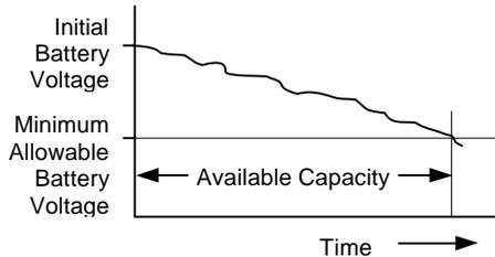
Figure 4: Relationship between voltage drop and battery capacity. The minimum allowable voltage is established by the battery manufacturer.
