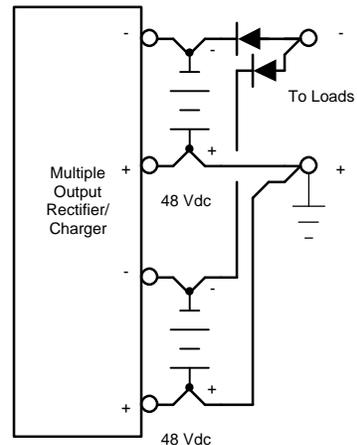
Figure 3: A rectifier/charger with multiple outputs provides better value since a common incoming step-down transformer and rectifier is utilized for all outputs. Not having to duplicate transformers and rectifiers save cost.
