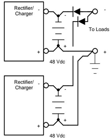
Figure 2: The traditional method of balancing the charge across a group of batteries to provide separate rectifiers for each battery string.
