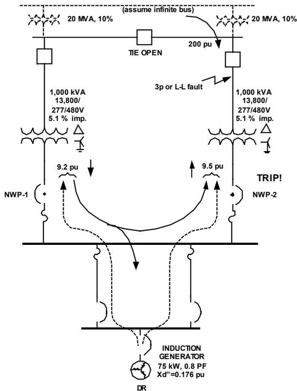
Fig. 1. Fault currents for primary fault, tie open
