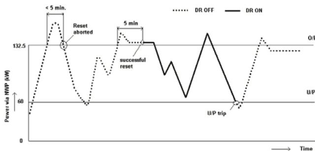
Fig. 8. System Deadband Operation
