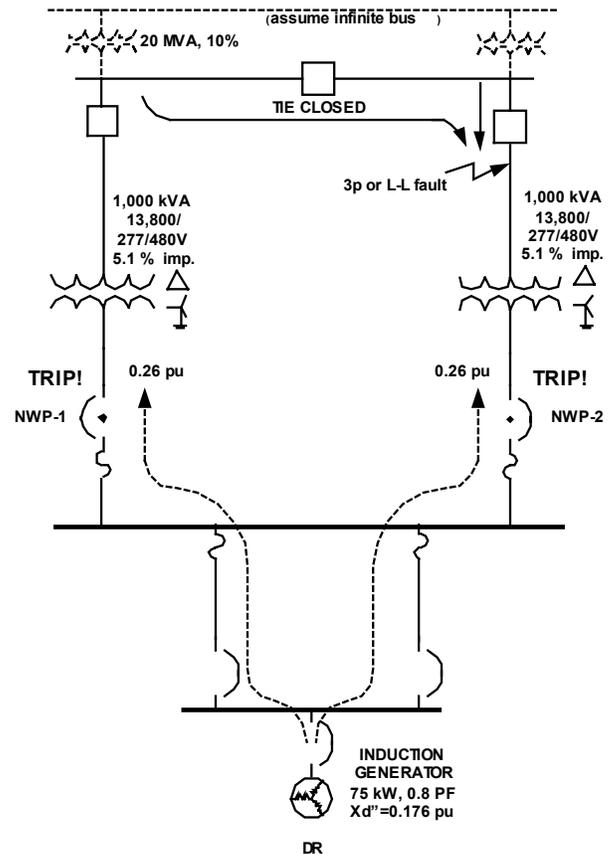
Fig. 2. Fault currents for primary fault, tie closed
