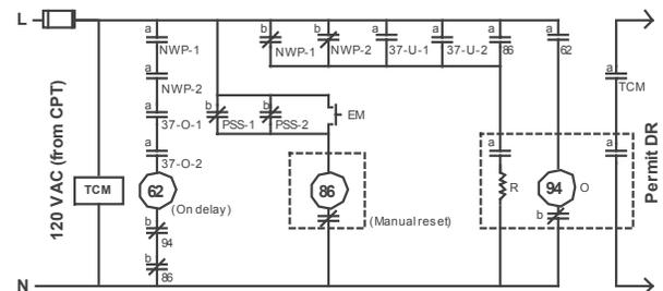
Fig. 6. Proposed Control Schematic of DR Control Circuit
