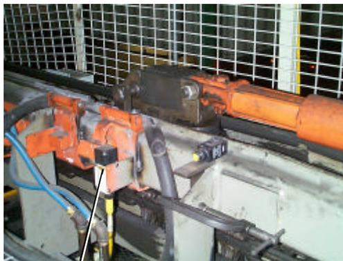
Limit Switch during actuation.
