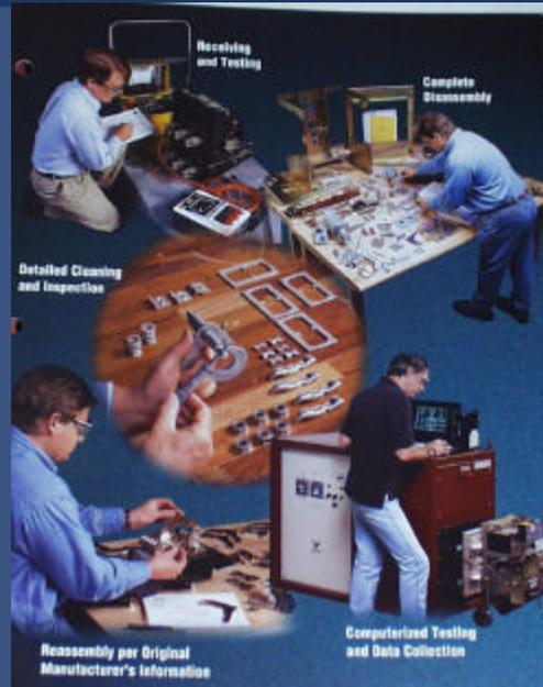
Even low voltage breakers can be brought to “like-new” condition using a technique known as “class 1 reconditioning”. In this technology the circuit breaker is disassembled to its smallest parts. Each part is inspected. Parts out of tolerance are replaced and acceptable parts are cleaned. The breaker is reassembled, tested to the industry standards and warranted. This is an option if new breakers are not available and you don’t want to replace the existing switchgear.
